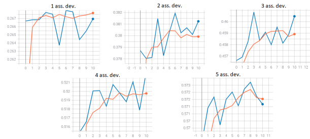
Fig. 8. The x-axis is number of trained epochs with y-axis being the accuracy. The blue line on all graphs are the accuracy for validation data-set, while the orange is the accuracy for the training data-set. These 5 graphs each show the accuracy for predicting the next assistive device among top 1, 2, 3, 4 or 5 devices.
